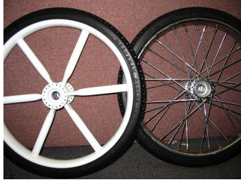
Welded Steel Mag Wheels / Standard spoked rear wheels
